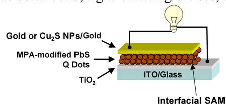
Figure 1. Device schematic of a solar cell based on PbS quantum dots.
