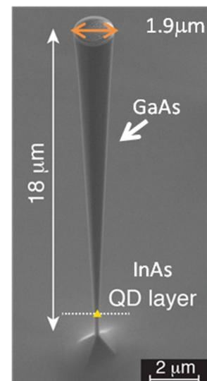
**Fig. 1. Scanning electron micrograph of the photonic nanowire.**
