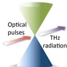
Fig. 1: Interband emission from optically excited graphene.
