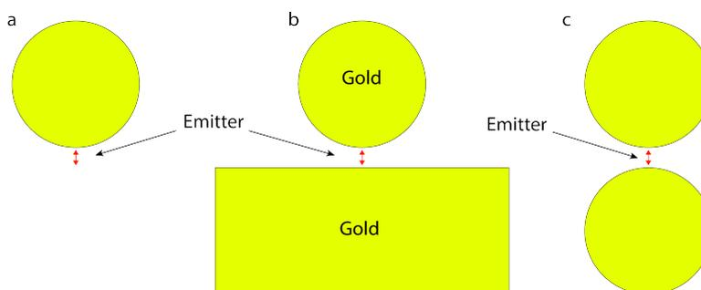
Figure 1. Schematic of the foreseen simulations. A single emitter (electric or magnetic) is coupled to **a.** a gold nanoparticle, **b.** a gold nanoparticle-mirror cavity, and **c.** a gold dimer.
