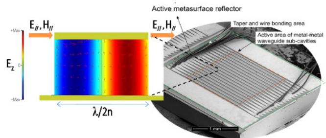
**Meta-surface geometry.** Resonator array integrated with THz QCL for vertical based THz amplifier (figure source: L. Xu et al, Appl. Phys. Lett. 107, 221105 (2015)). Inset: **Schematic of wavelength dimensioned resonator.** A 1D metal-active region-metal 1D resonator with size  $\lambda/2n$  supports a fundamental mode that radiates vertically as a dipole
